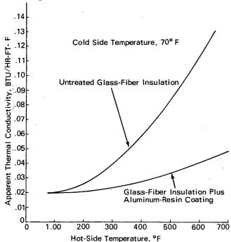
threefold or more, at a temperature difference of 600° F or greater between the outer insulation faces. The decrease results from impeding the transmission of radiant energy without increasing the solid conductance of the material. When large temperature differences exist between the outer insulation faces, such radiant energy represents a large portion of the total energy transferred.
