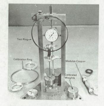
ASTM designation D-2290-64T) as the test specimen. Previously, elastic modulus determinations were
