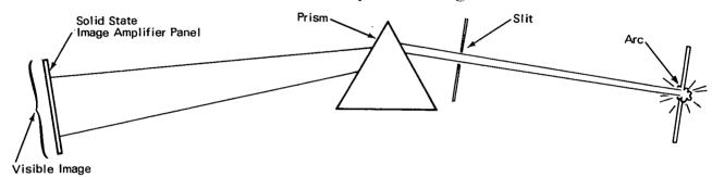
Relatively inexpensive, solid state image amplifier panels (see Ref.) can be used with simple spectroscopes over a range of wavelengths extending from the infrared (IR), through the ultraviolet (UV), and into the X-ray regions.
