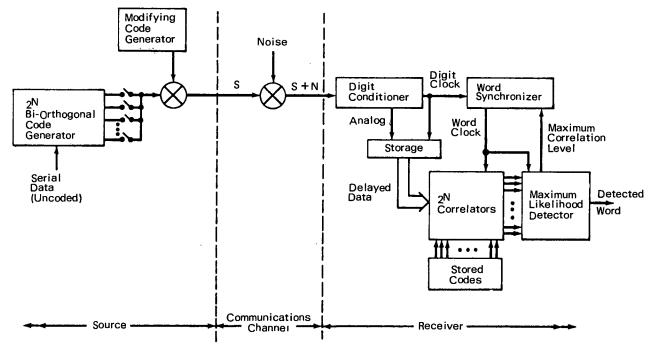
telemetry system for long distance communication consists of an airborne source, a gaussian additivenoise channel, and a ground receiver unit (see fig.). The airborne unit receives a random binary signal from the aircraft data handling subsystem and transforms it into a bi-orthogonal code. This code is modified by a self-synchronizing code, and the result is a binary code which needs only a single communication channel without additional bandwidth for word synchronization information.
