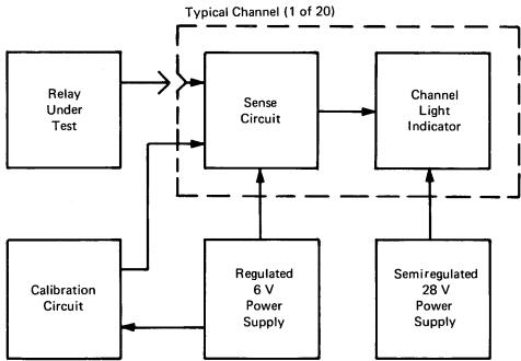
Relay chatter occurs when vibration momentarily opens contacts that should remain closed. The new detector compares the duration of such unwanted opening to a calibrated standard and lights an indicator if the standard is exceeded. The prototype unit indicates a failure if the contacts under test remain open for more than 10  $\mu$ sec. Each of its 20 sense channels can be individually adjusted to the standard by comparing the channel to an integral calibration circuit.
