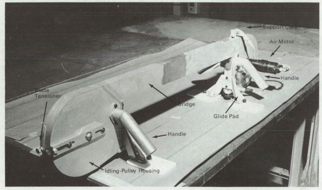
izontally. With coordination of the saw's vertical and horizontal movements, the blade can cut at any angle between these directions.
