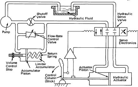
draulically actuated servo system to provide the operator with a realistic feel of column reaction in an actual aircraft. However, in the event that a large step function or a hard-over signal is applied by the servo system, the control column may be slammed toward the operator with sufficient energy to injure him.
