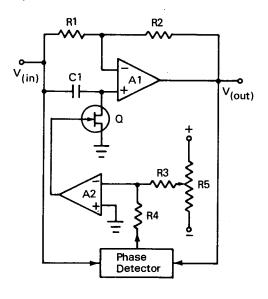
The new circuit includes a field effect transistor (FET), Q, operational amplifiers, A1 and A2, and a phase detector. The phase difference between the input and output is converted into a voltage which drives the electronic components of the circuit in such a way as to maintain the desired phase shift; i.e., the circuit is constantly in a balanced or null condition at a selected input-output phase relationship.
