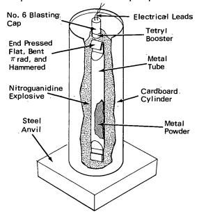
Set-Up for Explosive Compaction of Metal Powders and the elimination of incongruous effects which sometimes attend incomplete particle fusing may permit this technique to be applied to the large scale fabrication of intermetallic compounds with specifically formulated characteristics; e.g., semiconduction, superconduction, or magnetic properties. This method of synthesis should prove valuable to industries engaged in pyrometallurgy and materials fabrication.
