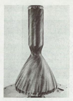
Graphite Mandrel with Tungston Screen Assembled sten, which is accomplished by reducing tungsten hexafluoroide,  $WF_6$ , with hydrogen,  $H_2$ :  $WF_6 + 3H_2 \rightarrow W + 6HF$
