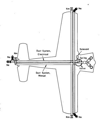
time required to effect any changeover in the current systems is altogether too long to permit the pilot to switch from one mode of operation to the other in emergencies, and there is a reluctance of the pilot to depend on all-electric systems, it became necessary to seek an improved attitude control system.
