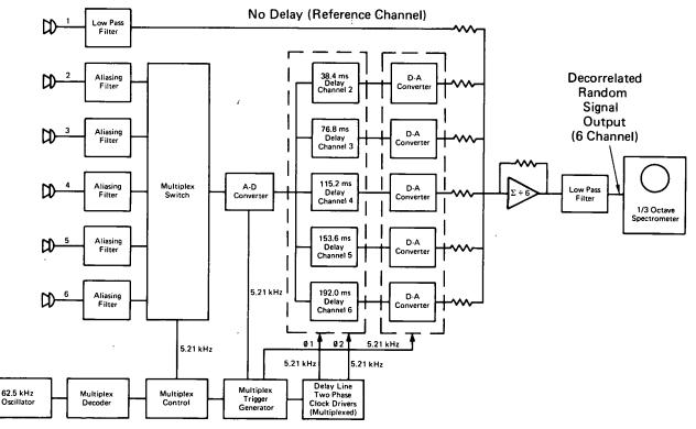
Because of the transmission characteristics of a reverberation room, the sound pressure level in the room is a function of measurement position and frequency. Also, a large test object absorbs sound, distorting the field. These problems make it impossible to describe the sound field in terms of a single point of measurement.
