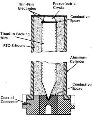
wafer in the shape of a conical frustum. The overall transducer is approximately 0.32 cm (1/8 in.) in diameter and 3.81 cm (1.5 in.) in length. The piezoelectric sensing element, a 0.051-cm (0.020-in.)-thick crystal of lead zirconate titanate, is cut as a conical frustum having base angles of 1.31 radians  $(75^{\circ})$ . This geometry was selected in order to ensure
