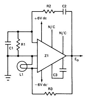
and do not exhibit the low power consumption, portability, simplicity, and drive capability achieved with this design. The oscillator, due to its low cost and high performance, has application as a loudspeaker tester and an audible alarm (when connected to a loudspeaker), as well as in laboratory and field test generators, and in timing generators.
