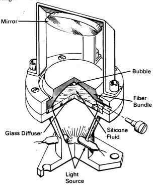
gular position indicator because it is simple, rugged, and small in size, and is impervious to the effects of temperature and vibration.
