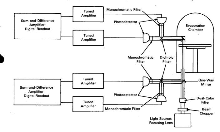
An improved dual-wavelength system (see fig.) monitors the fabrication of high-quality optical filters and other highly precise film deposition operations. Single-wavelength monitoring systems lack the required degree of accuracy. Dual wavelength systems were designed to generate the output signal of an element that would change rapidly at the point when the deposition process should change or stop.
