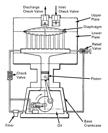
causes the diaphragms to flex, alternately drawing the gas into and discharging the gas from the cavities above the diaphragms. The diaphragms are clamped between bolted upper and lower plates and serve as their own gaskets.
