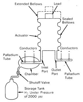
As shown in the schematic diagram, the conceptual actuator consists of a sealed bellows which is provided with inlet and outlet ports. A supply of hydrogen under pressure (typically 2000 psi) is contained in the storage tank. The tank is connected by tubing and a shutoff valve to a chamber completely enclosing a
