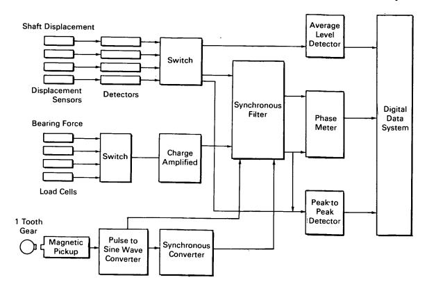
A digital data acquisition system has been developed that facilitates the recording of steady state and dynamic data of bearing and shaft displacement.
