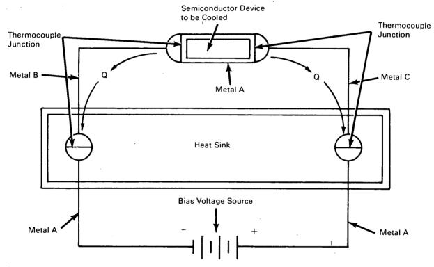
Thermocouple junctions made of bimetallic thin films have been incorporated into the active region of certain solid-state circuit components to improve their heat dissipation characteristics. These junctions use the Piltier effect to remove heat, with the electric current itself providing the heat transfer medium.
