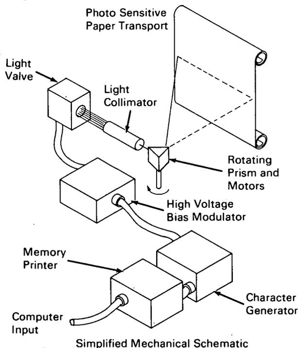
This new conceptual design for a high speed computer printer uses a Kerr cell as a light shutter for controlling the print on photosensitive paper. Applied to output data transfer, the information transfer rate of graphic computer printers could be increased to speeds approaching the data transfer rate of computer central processors (5000 to 10,000 lines per minute).
