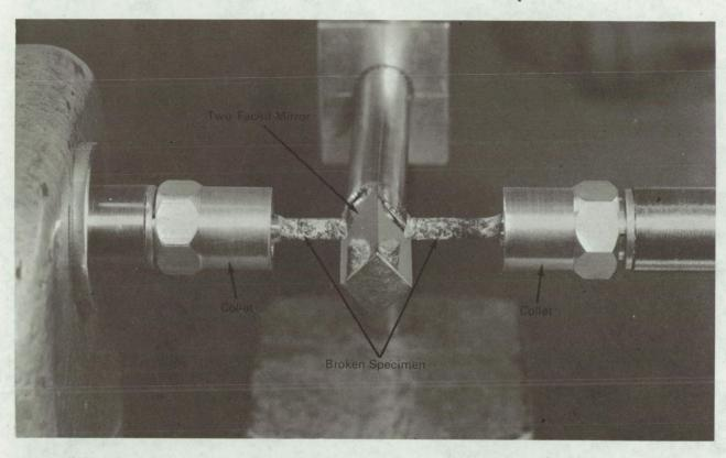
A small broken specimen can be reassembled without relative rotation of the faces of the fracture. The cemented fracture can then be sectioned metallographically, for example. One such technique was designed for reassembly of a 0.125-in.-diam specimen broken during stress-corrosion tests.
