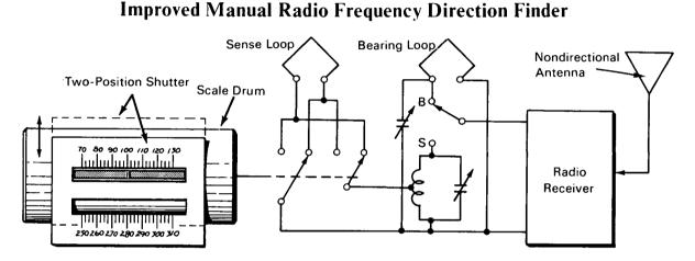
The standard procedure for taking a bearing on a radio signal is to rotate an antenna loop direction finder until the received signal intensity is minimal. The ordinary rotating loop direction finder indicates two bearings  $-180^{\circ}$  apart — when the loop is rotated through one complete cycle. The conventional method of determining which is the true bearing introduces possible error due to misjudgement of the signal intensity and requires two complete rotations of the loop.
