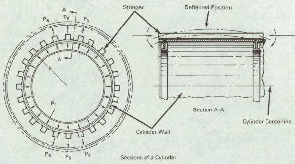
A new method accounts for the skin's hoop restraint on the beam-column behavior of an axially loaded, stiffened, cylindrical shell; each stringer is treated as an independent column on an elastic foundation. For the very conservative former method it was assumed that the stringers were radially supported by the frames only, which resulted in either overweight structures or unrealistically low margins of safety.
