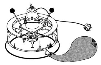
A portable universal router, as shown in the drawing, could perform such tasks as cutting holes of large diameter and irregular shapes, machining recesses, and drilling holes with certain edge-distance limitations. Mounted perpendicularly above the workpiece is a high-speed electric router motor. The motor housing is mounted on the top of a cylindrical tool housing which rests on the workpiece. The housings are coupled so that the router may be moved in the x-y plane.
