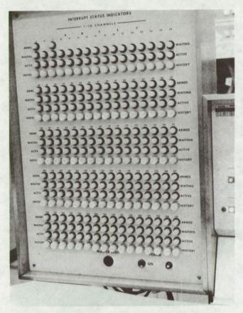
This digital computer programming aid provides a means of visual information which enables an operator to debug computer programs during program check-out. Previously, an operator often had to dump core, and trace the program until the error was found, consuming a good deal of time and increasing the probability of human error. By means of interrupt status indicators, the operator can debug his program during
