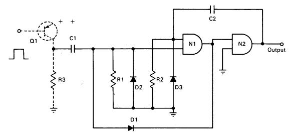
The illustrated circuit represents a design improvement in one-shot multivibrators. A breadboard model has been tuned to produce output pulses from one microsecond up to several seconds in width, with up to a 95% duty cycle, and with lower power consumption than is possible with previously existing circuits.
