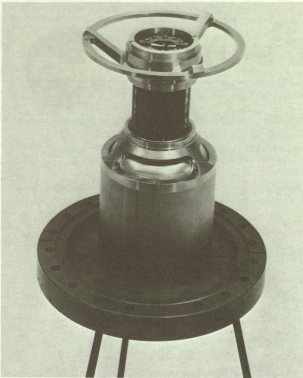
Figure 2. Hydrogen Maser Atomic Source Mounting Array
