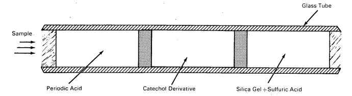
A colorometric method has been devised for the detection of very low concentrations of ethylene glycol vapor in air or other gases. Ethylene glycol is a common antifreeze and industrial solvent; its vapor is toxic at relatively low concentrations. Thus a simple quantitative test for this vapor would be useful in detecting leaks from systems containing the fluid.
