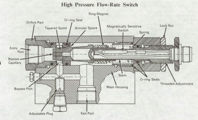
A reliable high pressure flow-rate switch of a new design adjusts easily over a wide switching range and operates uniformly over many cycles. It should find ready acceptance in commercial hydraulic applications.
