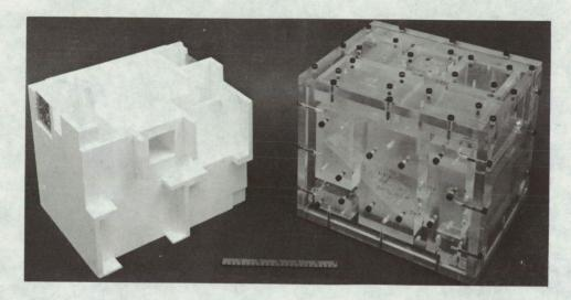
Clear acrylic sheet may be used to construct molds for fluid elastomers that are cured or vulcanized at room temperature. This technique offers the advantage of easier machining, compared to metal, and the ability to see through the mold and thus ensure that all cavities and corners are filled during the injection process.
