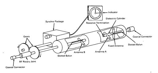
This innovation is an accurate radio frequency attenuator having negligible insertion loss at minimum attenuation. It can be used for making precise antenna gain measurements.
