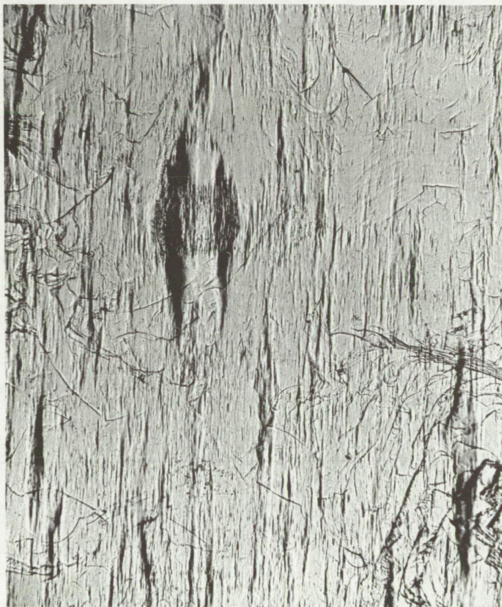
Cleaved basal-plane surface of pyrolytic carbon deformed by tension (times 100)
