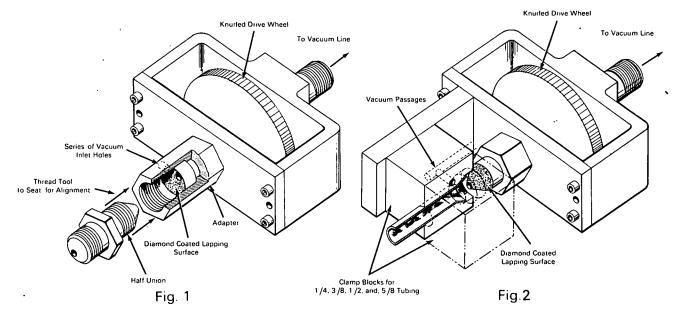
A portable tool has been designed in two versions, one for repairing the seats of tube fittings (half unions) and the other for repairing the flared ends of tubing. Each version operates on a like principle, that of lapping to remove imperfections from tube and fitting interfacing surfaces.
