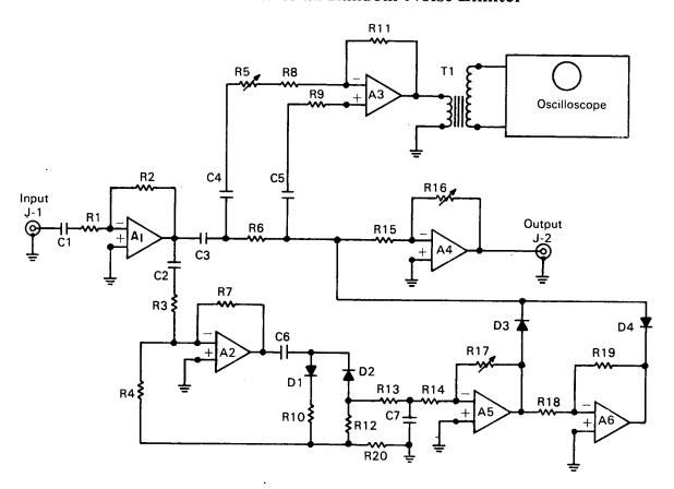
This circuit has been designed to limit the positive and negative peaks of a random-noise signal. Limiting is held to a value not exceeding 3 times the rms value of the random-noise signal. The circuit can be used to limit the peak acceleration automatically and continuously during random-noise vibration testing to a value no greater than 3 times the rms acceleration level.
