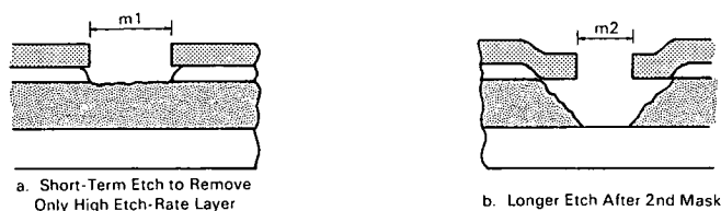
Fig. 2. Multiple Masking, Technique 1
