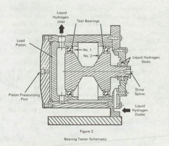
Use of large-bore, liquid hydrogen-cooled, ultrahighspeed, rolling-contact bearings of an optimum design allows optimization of large rocket engine turbopumps in which bearing speed is a limiting factor. Extensive information is now available on these bearings.
