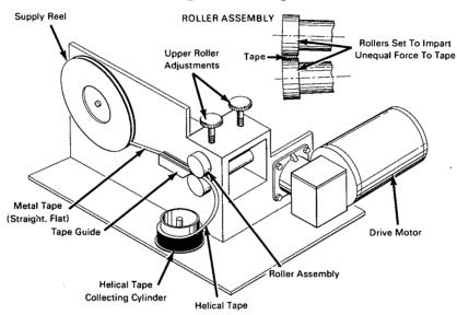
When thin metal tapes are wound into helical coils by the edge forming technique, the inner edge of the tape tends to buckle and corrugate. As coil diameters are decreased or tape width increased, corrugation distortion increases. Successful use of this method is limited to relatively thick metal tapes with a small width-to-thickness ratio.
