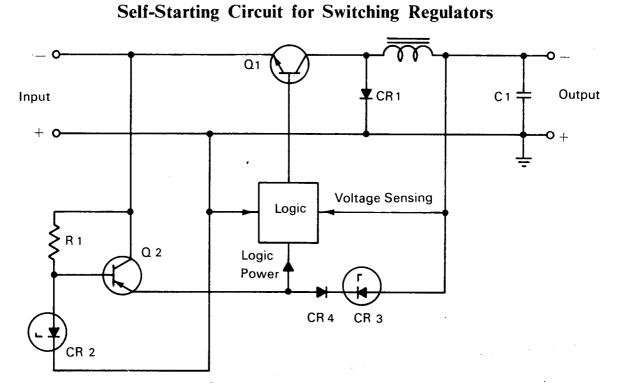
Switching type regulators which use a logic circuit to sense a change in output voltage and provide a correction signal for dc power sources are being used in an increasing number of applications.
