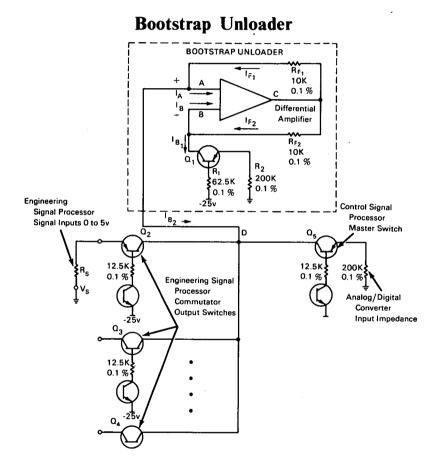
A circuit has been invented that can sample a number of transducers in sequence without drawing current from them. Novelty in the invention consists in the use of a differential amplifier with one input connected to a circuit which is the equivalent of the circuit to be unloaded. In this configuration, the other input delivers the proper unloading currents.
