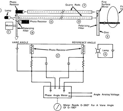
the rod to the flow vane's rotatable disc (E). This disc consists of a plastic polarizing filter bonded to a mirror surface. The flow vane rotates disc (E).
