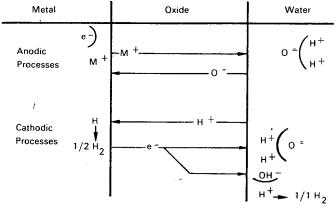
An electrochemical study of aluminum corrosion in boiling high-purity water has been reported. An equation relating current and electrochemical potential was derived on the basis of a physical model of the corrosion process.
