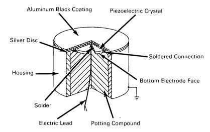
A transient-heat transfer gage has been developed to measure the total radiation intensity from vacuum ultraviolet (below 1200 angstroms) and ionized high-temperature gases. Available metal thin-film or pyroelectric gages cannot be used for such measurements. The surface of the thin-film gage is shorted, and the surface electrodes of the pyroelectric gage are penetrated by vacuum ultraviolet photons, causing noise and depolarization of the sensor crystal.
