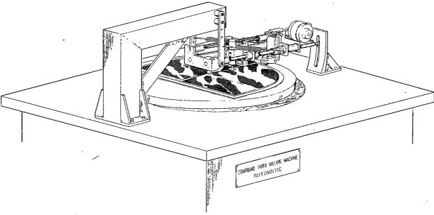
A milling machine has been designed to taper panels from a common apex to a uniform height at panel edge regardless of the panel perimeter configuration. While this can be done by expensive and sophisticated equipment having at least 3-axis motion, the subject device is simple and cheap to construct and operate, performs efficiently, and can be automated.
