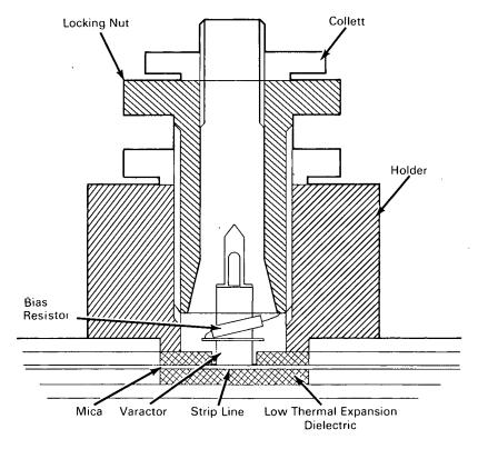
A device has been designed that improves the performance of a stripline varactor harmonic multiplier by providing means for positioning the varactor diode with respect to the stripline circuit so that series resonance of the diode is obtained. The innovation also reduces detuning effects, due to thermal expansion, over a wide temperature range.
