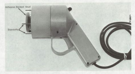
This tool will facilitate the bonding of thermoplastic-backed studs to smooth, hard surfaces (such as marble). Such studs can be used for mounting loads, such as heavy pictures or signs, on walls in public buildings where defacement with drilled holes cannot be tolerated. These studs can easily be removed, when desired, by softening the plastic bonding with heat from the gun.
