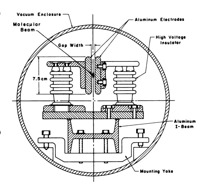
Figure 7. Cross-section of electrode assembly.
