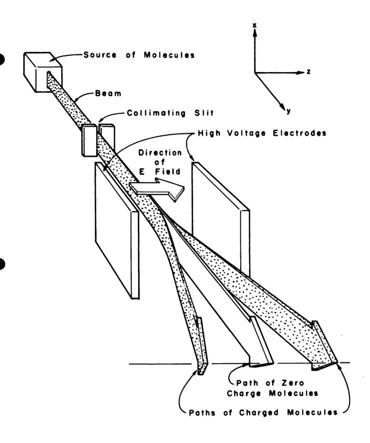
Figure 2. Molecular beam measurement of atomic or molecular charge.
