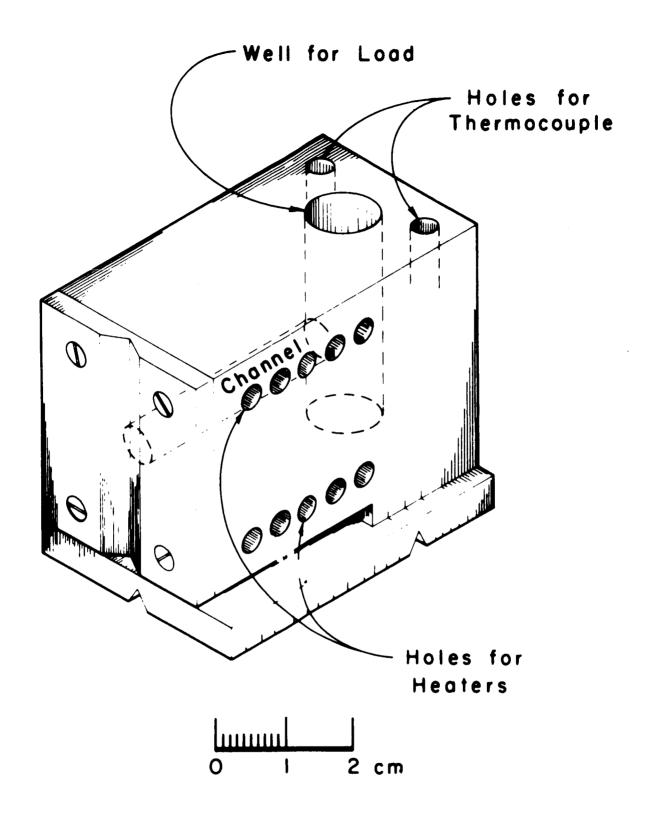
Figure 5. Conventional oven used for alkali atoms.
