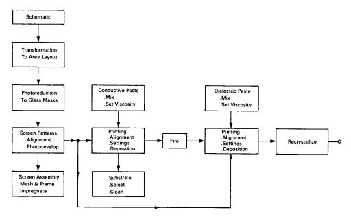
In the past, screened hybrid microcircuits have used low dielectric thick films for capacitors. These consist of ceramic dielectric particles mechanically suspended in a lead monosilicate glass matrix. Because of the small volume of high dielectric particles (35% by weight) which can be packed into the low dielectric glass, the dielectric constants of such thick films are less than 100. The mechanical suspension results in low-density structures featuring high-dissipation factors.
