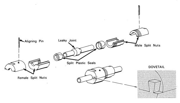
Prior methods of repairing leaking tube joints involved replacement of the soldered joint. This entailed removal of the union by debrazing or by machining and necessitated system flushing, purging, and recharging.
