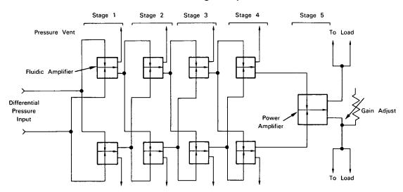
A five-stage, high-gain, push-pull fluidic amplifier has been designed to provide increased range and improved linearity compared to previous fluidic amplifiers.
